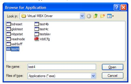
By default, the test4.exe is located in \Program Files\Cyberlogic\Virtual MBX Driver directory.
