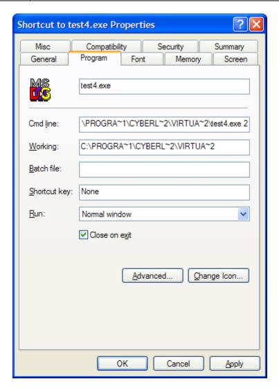
Append command line switches, if needed, in the *Cmd line* field.
